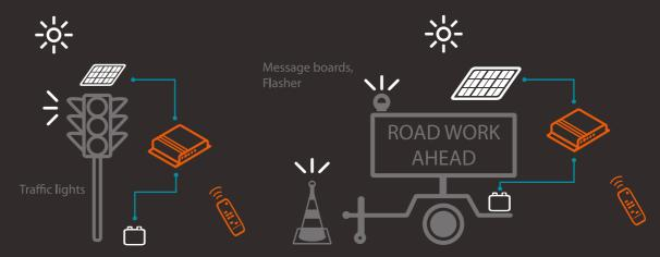
Solar powered traffic control systems are energy-saving and eco-friendly solutions that contribute to road safety. The robust and waterproof housing, compact size, and high efficiency of the CIS-MPPT makes it the perfect choice for all types of outdoor applications.
