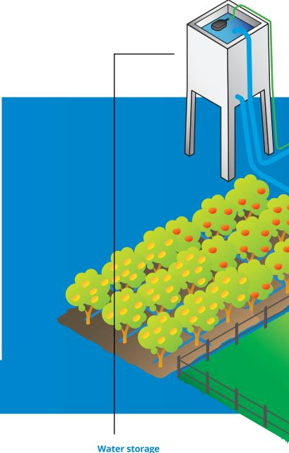
Introducing water storage to a solar water pumping system allows for increased seasonal demands to be met, or simply for overnight water availability without a generator or grid power.
