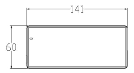
The model AP-FN90-12 charger by natural air. The input voltage range is 100-240Vac, the single-channel voltage is up to 14.6V, and the maximum current is 6A. The power supply has reverse polarity protection. The entire power supply is designed in strict accordance with safety regulations.
