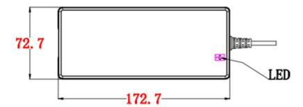
The model AP-PN120-24 charger by natural air. The input voltage range is 100-240Vac, the single-channel voltage is up to 29.2V, and the maximum current is 4A. The power supply has reverse polarity protection. The entire power supply is designed in strict accordance with safety regulations.
