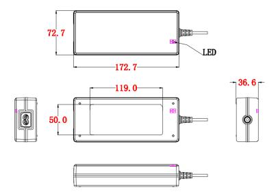
Tolerance of outline dimension is  $\pm 0.5$ mm, others are  $\pm 0.2$ mm in the diagram;
