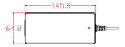
The model AP-PN180CH02400060 charger by natural air. The input voltage range is 100-240Vac, the single-channel voltage is up to 29.2V, and the maximum current is 6A. The entire power supply is designed in strict accordance with safety regulations.
