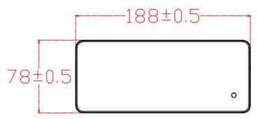
The model AP-PN240CH02400080 charger uses natural cooled charger. The input voltage range is 100-240Vac, the single-channel voltage is up to29.2V, and the maximum current is 8A. The power supply has reverse polarity protection. The entire power supply is designed in strict accordance with safety regulations.
