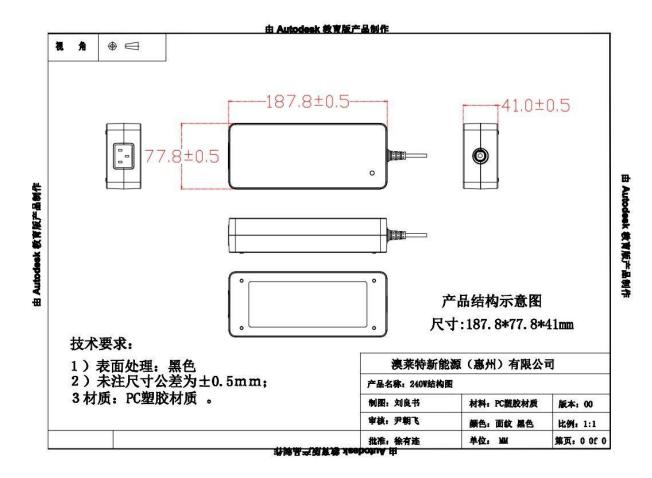
Tolerance of outline dimension is  $\pm 0.5$  mm, others are  $\pm 0.2$  mm in the diagram;
