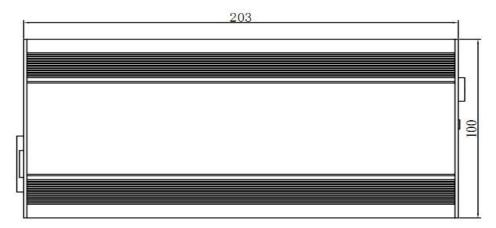
The model AP-PF360-24 charger is a fan cooling charger. The input voltage range is 100~240Vac, the single-channel voltage is up to 29.2V, and the maximum current is 10A. The power supply has reverse polarity protection. The entire power supply is designed in strict accordance with safety regulations.
