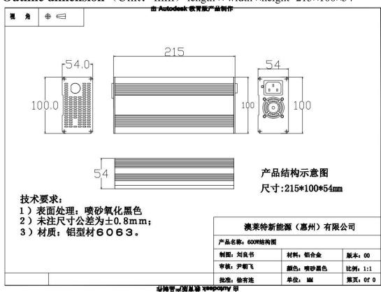
Tolerance of outline dimension is  $\pm 0.5$ mm, others are  $\pm 0.2$ mm in the diagram;
