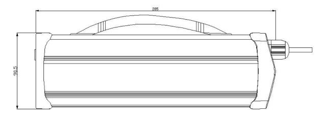
The model AP-PF900-48 charger uses an 80 \* 80 \* 20mm bearing fan-cooled charger. The input voltage range is  $100 \sim 240$ Vac, the single-channel voltage is up to 54.6V, and the maximum current is 15A. The power supply has reverse polarity protection. The entire power supply is designed in strict accordance with safety regulations.
