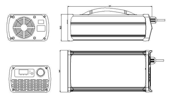
Tolerance of outline dimension is  $\pm 0.5$ mm, others are  $\pm 0.2$ mm in the diagram;
