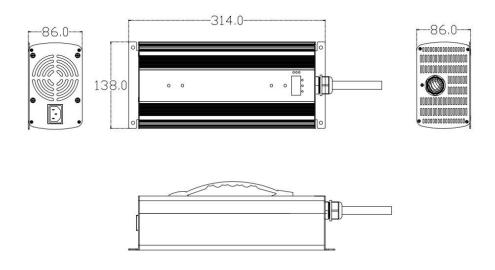
Tolerance of outline dimension is  $\pm 0.5$ mm, others are  $\pm 0.2$ mm in the diagram
