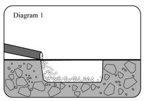
1. Dig a hole on ground and fill with proper amount of grout.
