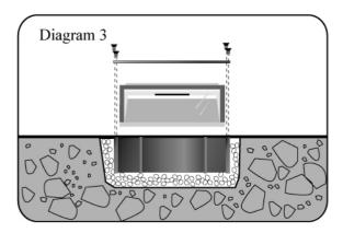
3. After the cement become dry, clean up cement that has filter into the mounting case, and then put light into the mounting box, and fix up it by cover the stainless steel on the mounting box and fasten it by stainless steel bolt.
