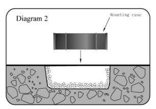
2. Put the mounting case inside the hole, and install on the same level as ground surface.
