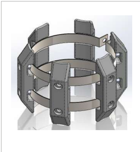
Figure 52: Sacrificial anode for submersible pump ends
