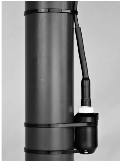
Figure 38: Well probe fixing
